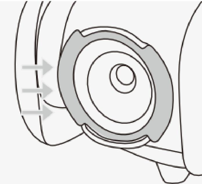
Align the magnetic ring with the drone's camera, press firmly to center and secure it, then ensure the tape is fully adhered by pressing both sides.
