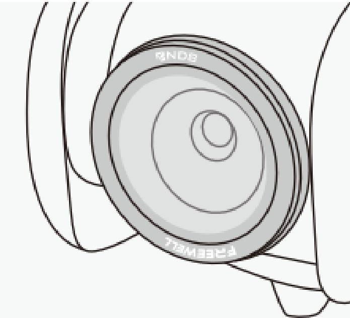
Once installation is complete, to replace the filter, simply remove the current filter and attach a new one. The magnetic ring remains in place, and you only need to replace the filter without removing the magnetic ring.
