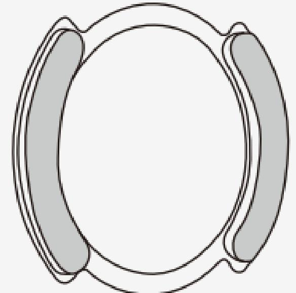
Remove the adhesive backing from both sides of the magnetic ring to expose the double-sided tape.
