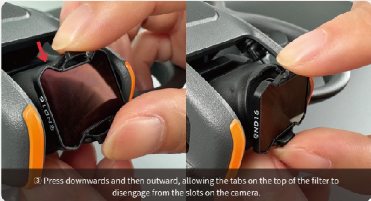
③ Press downwards and then outward, allowing the tabs on the top of the filter to disengage from the slots on the camera.
