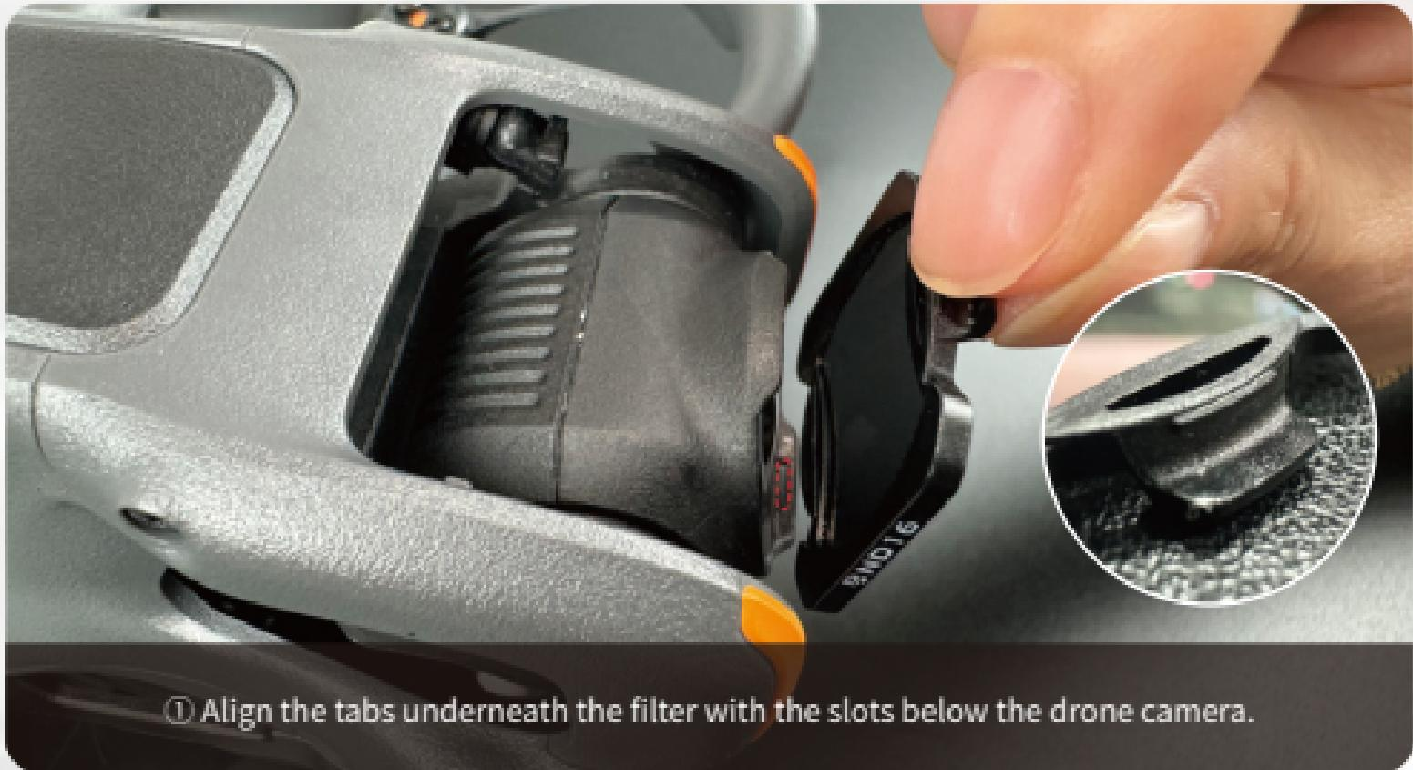
① Align the tabs underneath the filter with the slots below the drone camera.
