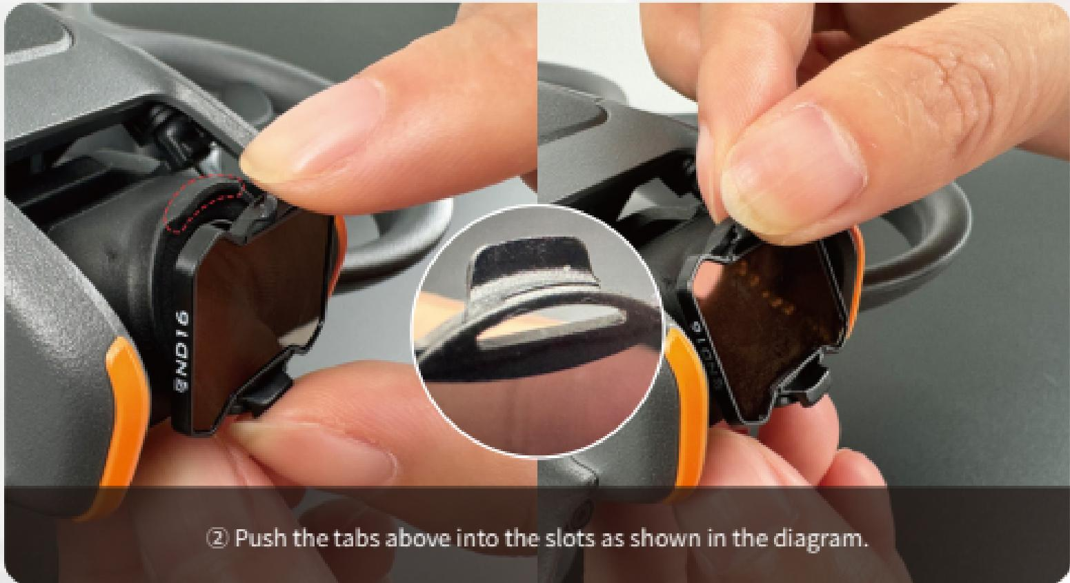
② Push the tabs above into the slots as shown in the diagram.
